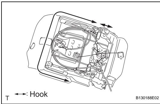
(c) Using a screwdriver, detach the hooks and remove the seat cushion cover (with pad) from the seat cushion spring.
