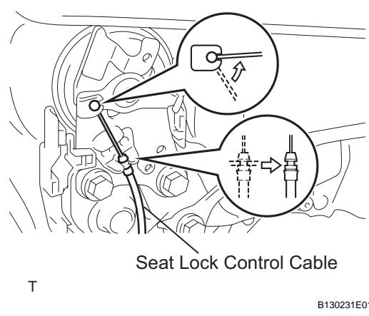
(c) Disconnect the seat lock control cable on the RH side from the seatback as shown in the illustration.
